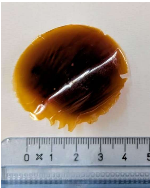
Figure 6.4 – Optical image of the aPPO film obtained by solution casting from a 5% wt. solution of aPPO in DMSO. The film shows good surface homogeneity and brown-translucent coloration.
