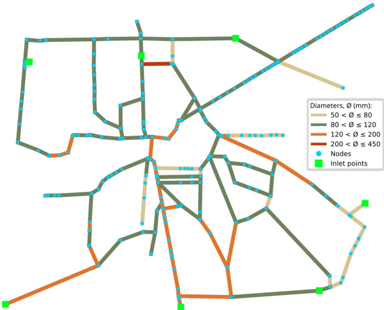
Figure 21. Diagram of the Real Network 1 water network. The diameter classes of the pipes are represented by different colors, while the nodes and entry points are indicated by blue circles and green squares respectively. Reproduced from Medio et al. (2024). [35]
