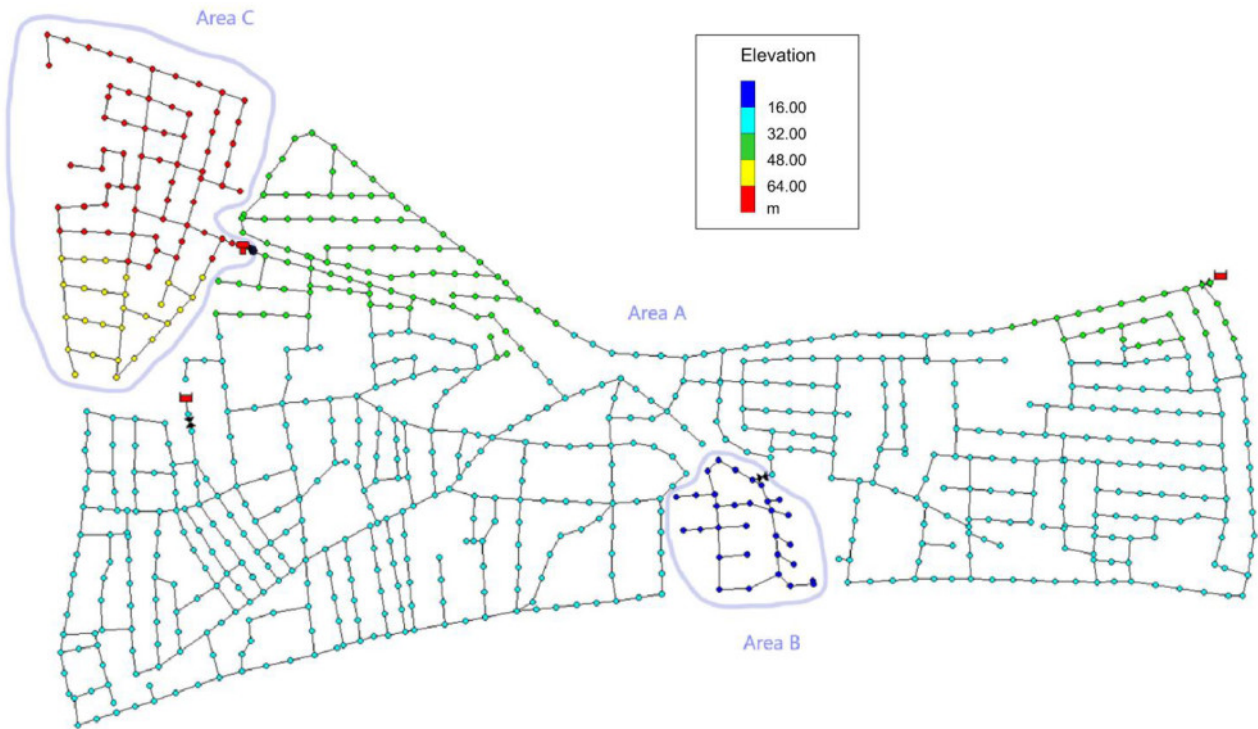
Figure 30. Reproduced from Vrachimis et al. (2022)[107]. Altimetric subdivision of the L-Town water network. Nodes are colored according to piezometric elevation, with increasing values from blue (16 m) to red (64 m). The network is divided into three macro-areas: Area B, corresponding to the lowest elevation and characterized by the lowest elevations; Area A, of intermediate elevation and morphologically central; and Area C, representing the highest portion. This altimetric distinction highlights the topographic variability of the system, useful for hydraulic analysis and monitoring planning.
