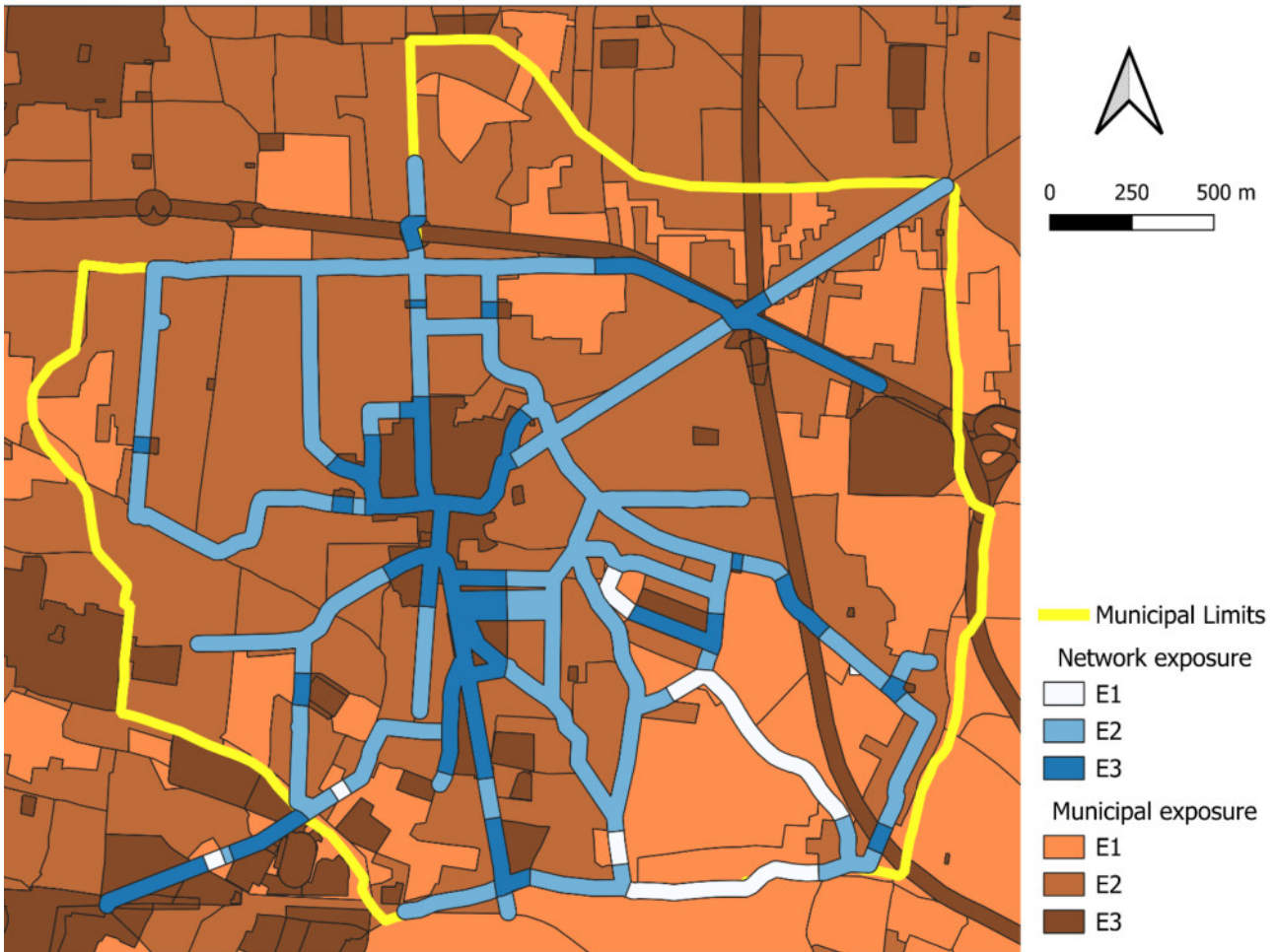
Figure 22. Zoning of territorial exposure (classes E1–E3) derived from the integration of ISTAT data, SIT and satellite observations. The pipelines inherit the prevailing exposure class of the area crossed, making it possible to distinguish the low (E1), medium (E2) and high exposure (E3) sections. The municipal perimeter is represented in yellow. Reproduced from Medio et al. (2024). [35]
