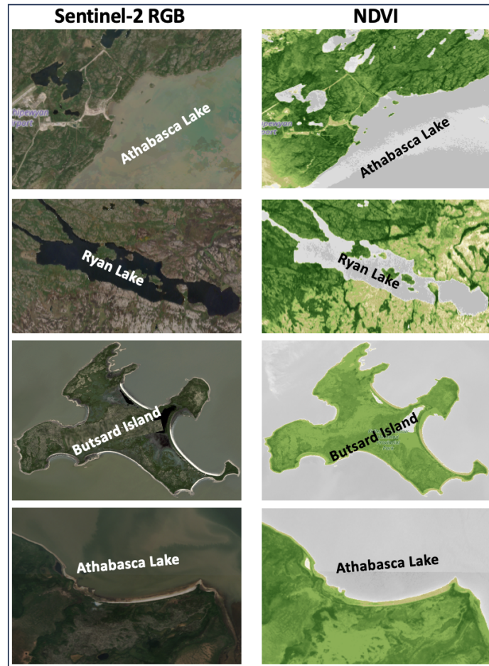
Figure 4.12 Comparative analysis of vegetated and sandy shorelines using Sentinel-2 RGB and NDVI data.
