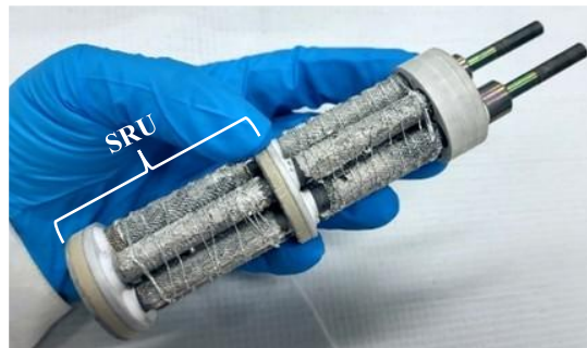
Figure 24. First tubular PCCEL stack prototype in PROTOSTACK project [71].
