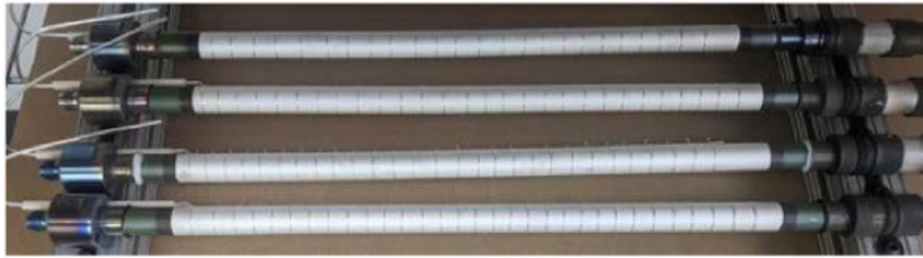
Figure 17. Tubular PCCEL tubes produced by Kee et al [59].
