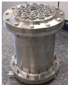
Figure 18. Tubular 1 kW PCCEL prototype developed in the Electra project [65].
