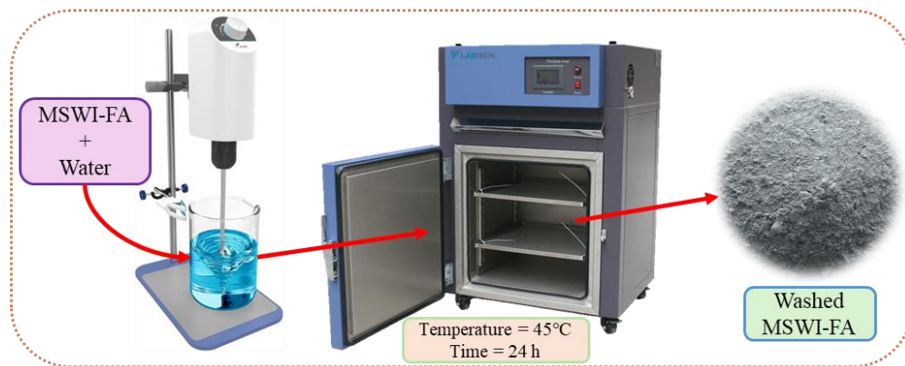
Figure 3.2 Illustrative diagram for MSWI-FA washing.
